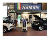
Thanks to the innovative hydraulic circuit, this ultra-modern station for recharging air conditioners can manage two different gases without having any contact between them. It is therefore possible to operate on two cars at the same time.
